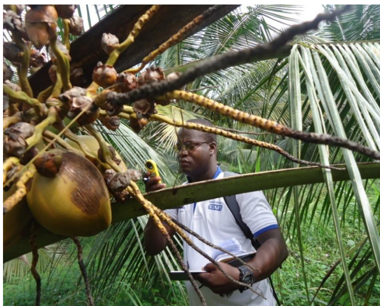
Figure 7. Using the Kestrel 2000 Anemometer to take readings of temperature, relative humidity and wind speed at the plantation.
