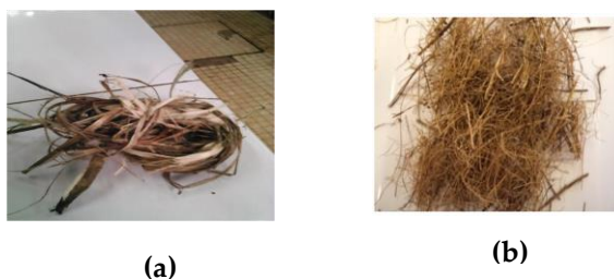
Figure 2. Kenaf fiber (a) and Date palm fiber (b) used.
