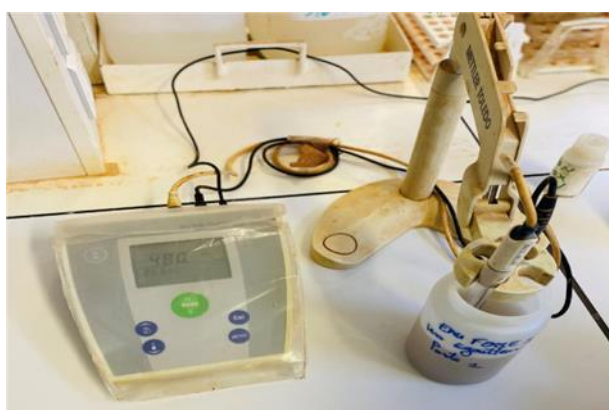
Figure 9. Electronic ORP meter used for oxidation reduction potential measurement
