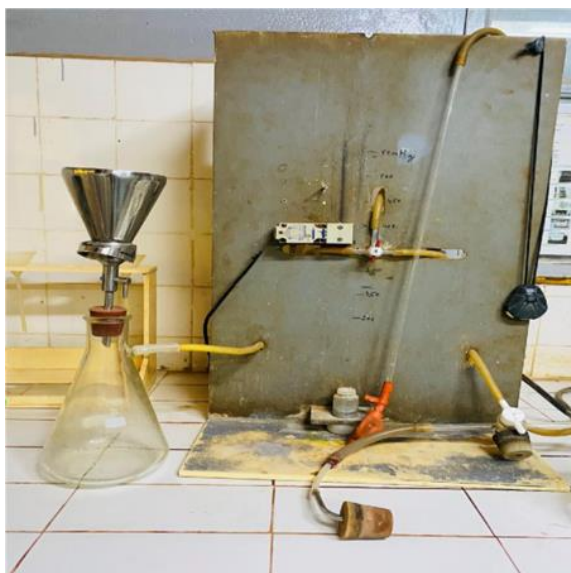
Figure 11. Filtration apparatus used for suspended solids concentration measurement
