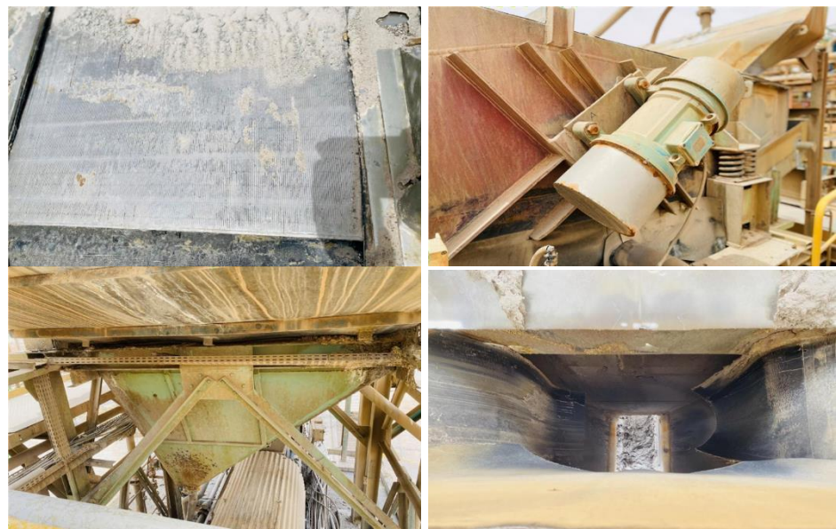
Figure 14. Operational components of the vibrating drainer and associated recycling equipment: (a) drainer screens or sieves, (b) drip motor, (c) water collection tank, and (d) sand recovery chute
