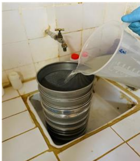
Figure 10. Passing the sample through the sieves for particle size analysis
