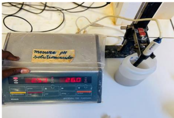
Figure 8. Electronic pH meter for pH measurement
