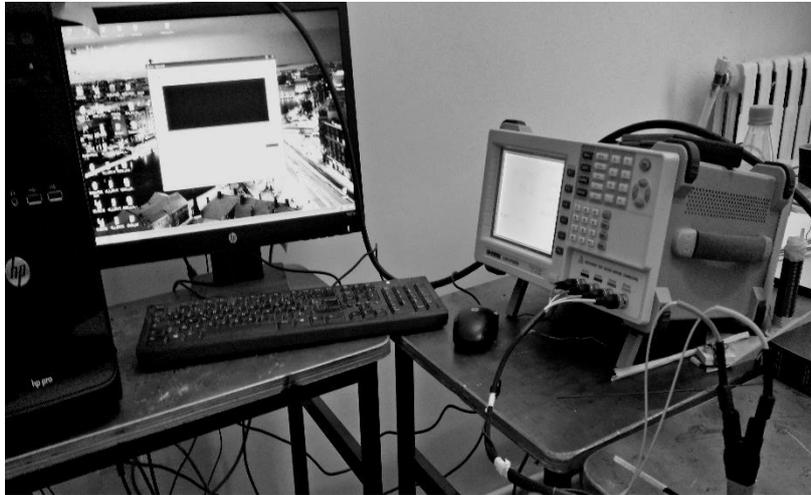
Figure 3. precision LCR-Meter
