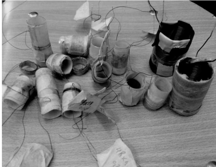
**Figure 1.** Fabricated coils with different winding topology
