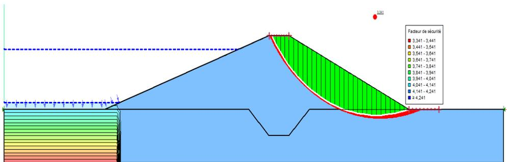
**Figure 9.** Stability Analysis during Rapid Drainage: Sliding Surface and Safety Factor (Downstream Slope)
