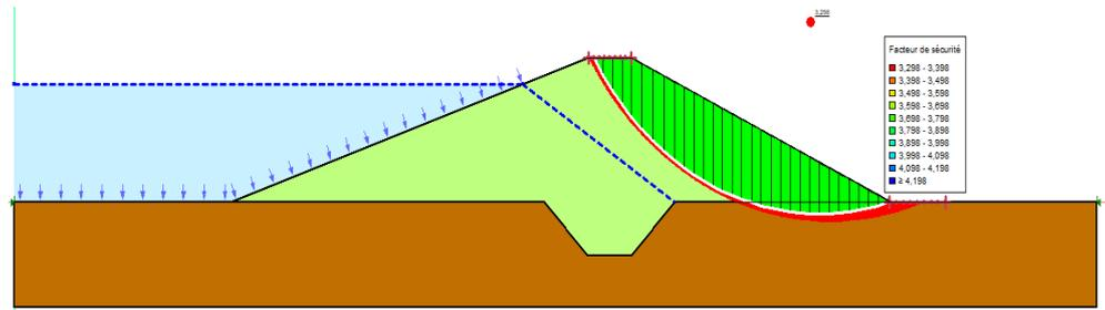
**Figure 7.** Stability Analysis under Normal Operation: Sliding Surface and Safety Factor (Downstream Slope)
