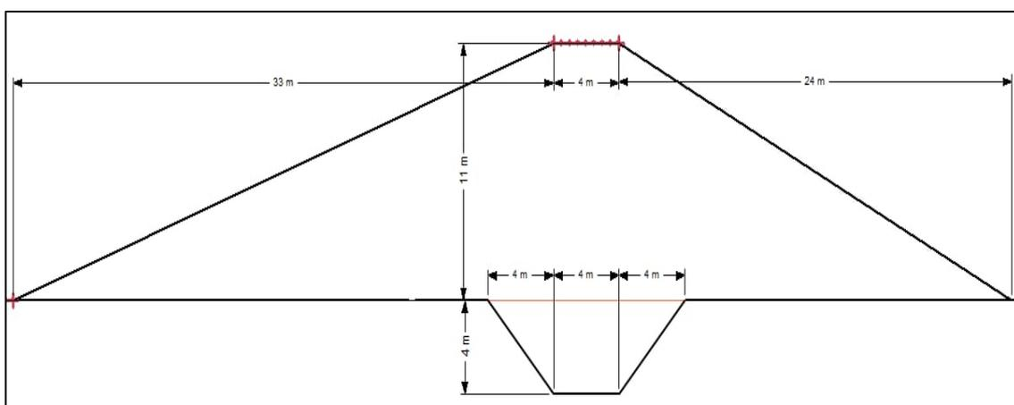
Figure 2. Geometry of the dike and arrangement of structural elements
