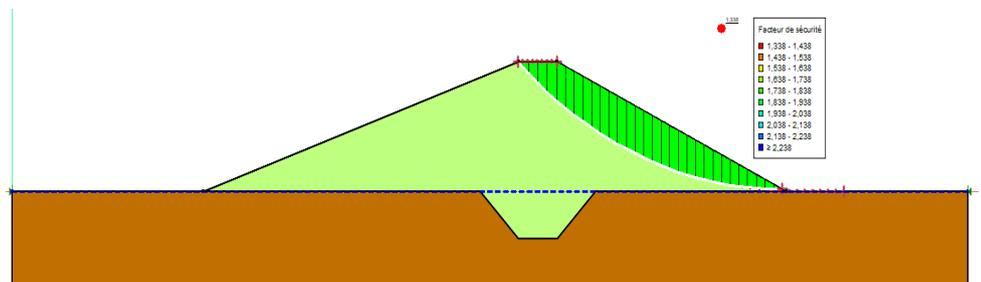
Figure 15. Empty phase stability analysis: sliding surface and safety factor (Downstream Slope)
