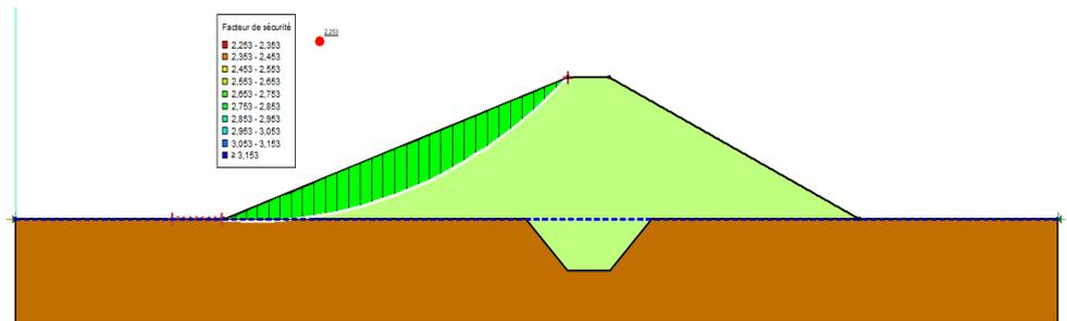
Figure 14. Empty phase stability analysis: sliding surface and safety factor (Upstream Slope)
