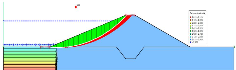
**Figure 12.** Stability analysis during rapid drainage: Sliding surface and Safety Factor (Upstream Slope)
