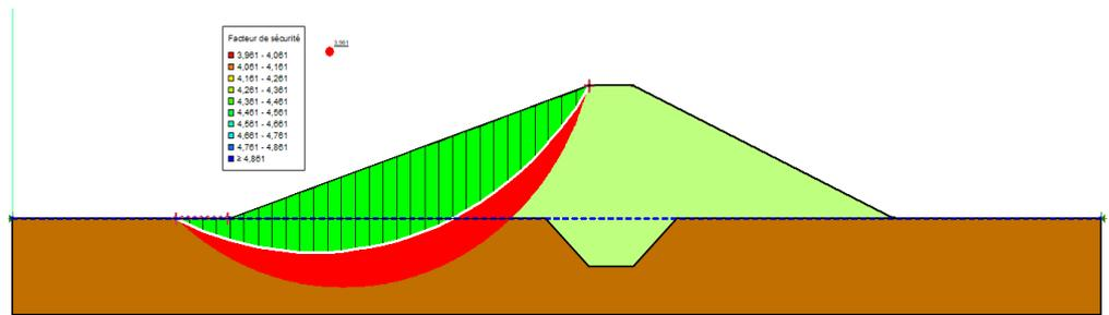
**Figure 4.** Stability analysis at the end of construction: Sliding surface and Safety Factor (Upstream Slope)
