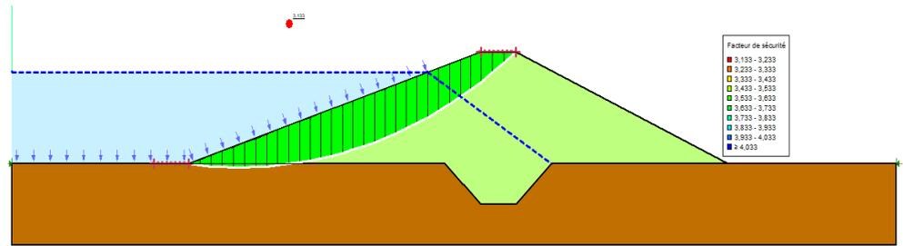
**Figure 10.** Stability analysis under normal operating conditions: sliding surface and safety factor (Upstream Slope)
