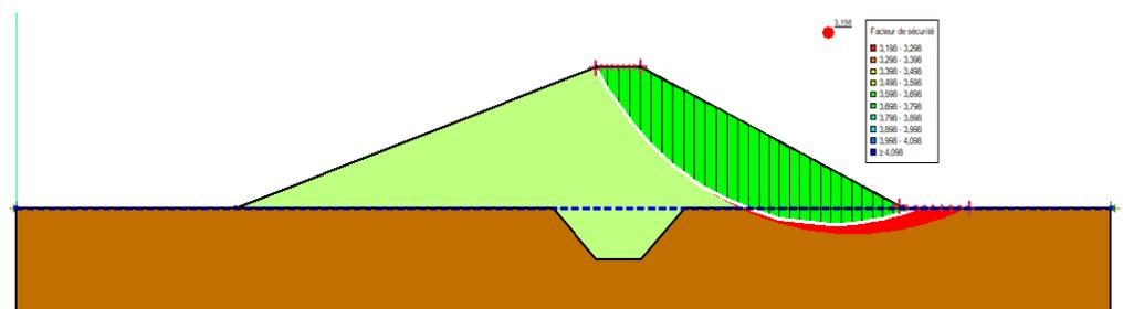
**Figure 5.** Stability analysis at the end of construction: Sliding surface and Safety Factor (Downstream Slope)
