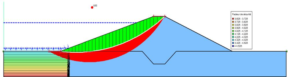
**Figure 8.** Stability Analysis during Rapid Drainage: Sliding Surface and Safety Factor (Upstream Slope)
