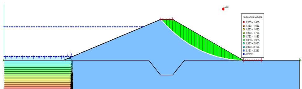
**Figure 13.** Stability analysis during rapid drainage: sliding surface and safety factor (Downstream Slope)
