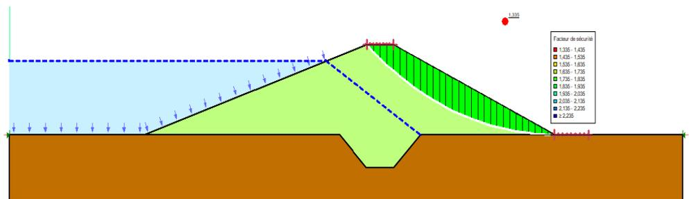
**Figure 11.** Stability analysis under normal operating conditions: sliding surface and safety factor (Downstream Slope)
