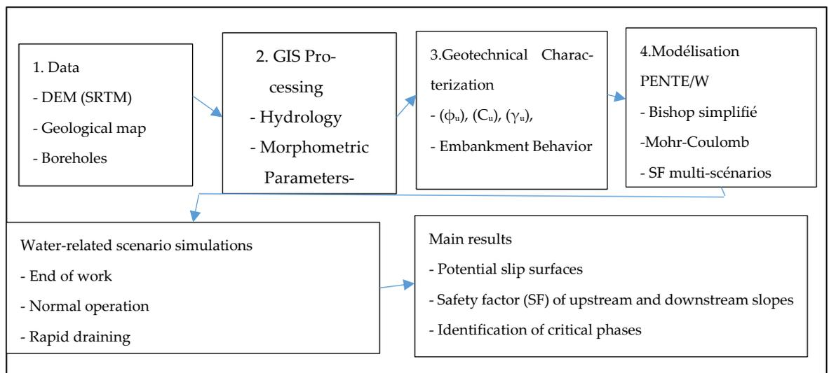
**Figure 3.** Methodological diagram for evaluating the stability of the Ayda wadi dike using a GIS-Geotechnical approach
