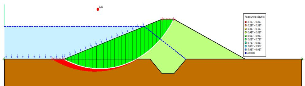
**Figure 6.** Stability analysis under normal operating conditions: Sliding surface and Safety Factor (Upstream Slope)
